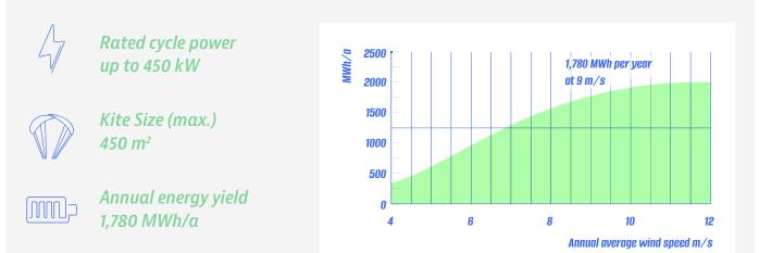
Single system, Standard Rayleigh wind distribution (k=2), Wind speed at flight altitude (300 m), Kite size: 450 m<sup>2</sup>, Tether length: 950 m, Air density = 1.2 kg/m<sup>3</sup>, 100 % Availability, 0 % Losses.
