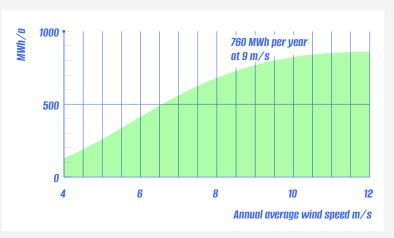
Single system, Standard Rayleigh wind distribution (k=2), Wind speed at flight altitude (200 m), Kite size: 170 m², Tether length: 800 m, Air density = 1.2 kg/m³, 100 % Availability, 0 % Losses.
